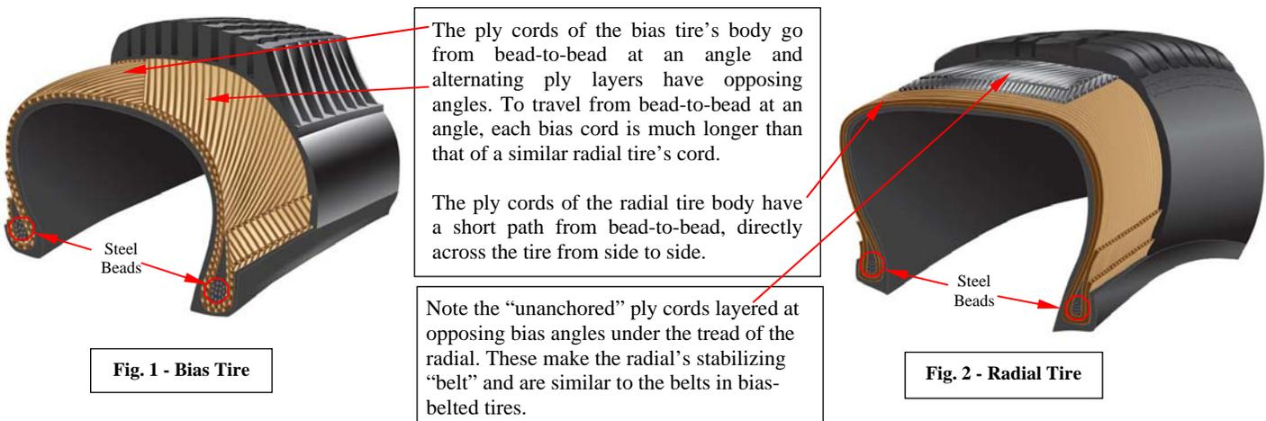
In a bias tire, plies always come in pairs so the angled cords in each ply are counter-balanced by the next ply's cords going the opposite direction (2 ply, 4 ply, 6 ply etc.). Bias ply layers create a much stiffer structure (like plywood's alternating wood grain layers) than a radial tire's body. If a sufficiently strong cord is available, a radial tire can operate with only one body ply and the cross-angled belt plies add stiffness only under the tread area.
